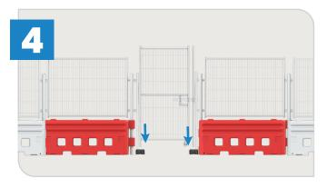
Locate the pedestrain gate and gate post, insert the gate into either of the remaining central rubber foot holes.
