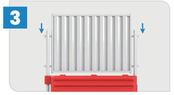
Lift a panel and hover it over the barrier, line up the brackets on the panel with the brackets on the posts.
