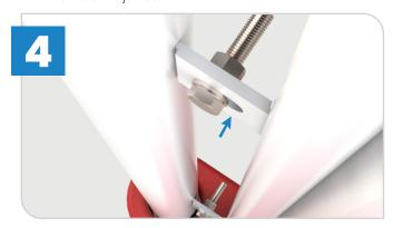
With one person on either side of the panel, push a M10 x40mm bolt with a washer on through each bracket and fit a washer and nut on to it the other side of the panel and secure with a impact driver.
