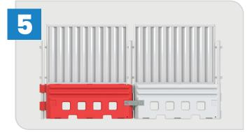
Once the fencing / hoarding panels are in place the RB22 Barrier system forms a robust boundary, with the extra panel also increasing the overall height to 2200mm.
