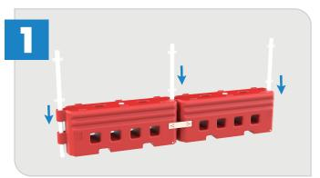
If using fencing or hoarding panels you will be supplied with metal connection posts instead of connection pins. Drop the connection posts in vertically through the holes where the RB22 barriers are joined.
