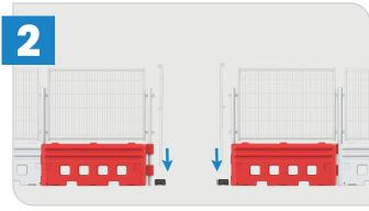
Locate 2x adaption posts and position one into each rubber foot, insert each post into the central hole closest to the RB22 barrier.
