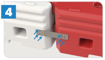
For added security and resistance place the face plate on each side of the barrier and fasten the 12 screws with an allen key. Bolts should never be overtightened, and never use a drill or impact driver as this may cause damage to the barrier.
