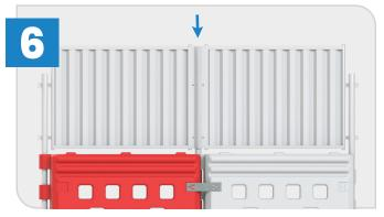
To install infill panels line up with brackets of the posts and panels on the outside face of the system. Do this at the same time as when the hoarding / fencing panels are installed, as the bolts must be threaded through the infill panel first.
