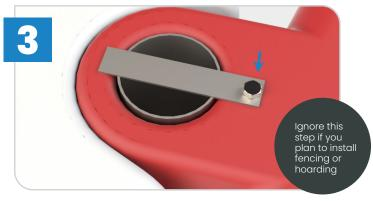
Secure the pin by screwing through the eyelet on top into the threaded hole situated next to the opening. Avoid using a drill / impact driver as this may cause damage to the barrier.
