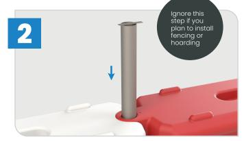
Next, insert the connection pin into the connection hole. Do NOT hammer this into place.
