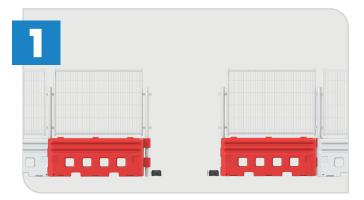
Locate 2x rubber feet and position one at each outer end of the already installed RB22 with mesh fence.
