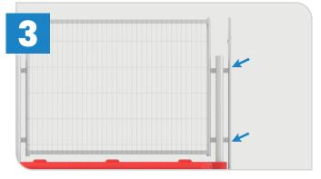
Connect each adaption post to each connection post using 2x M10 x 40mm bolts, washers and nuts on each side.
