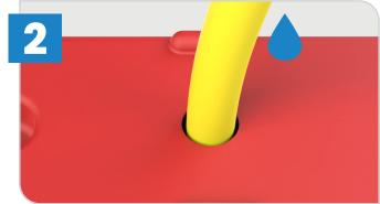
Once all barriers are securely set up, fill each barrier with water up to 540L. Once the barriers are full replace cap.
