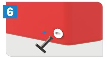
When it is time to dismantle the RB22's locate the release plug at the bottom of the barriers To unscrew and re-secure the release plug please use the 'T' shape key provided.
