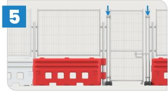
Connect the pedestrain gate and gate post to the adaption post using 2x couplers on each side.
